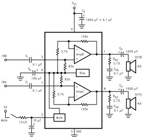
FIGURE 1. Typical Audio Amplifier Application Circuit
