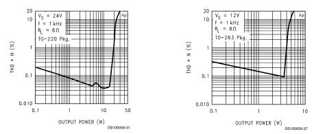
FIGURE 5. THD+N vs  $P_{OUT}$  for Bridge-Mode Application
