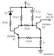
FIGURE 6. External Undervoltage Pull-Down
