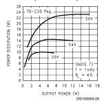
Power Dissipation vs Output Power
