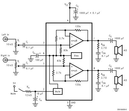
FIGURE 3. Circuit for External Components Description
