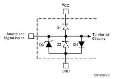
FIGURE 1. ESD Protection Input Structure
