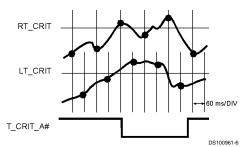
FIGURE 3.  $\overline{T\_CRIT\_A}$  Temperature Response Diagram
