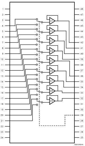
FIGURE 6. Block Diagram of LMC6009
