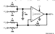
Where:  $V_0 = V_1 + V_2 - V_3 - V_4$  $(V_1 + V_2 \ge (V_3 + V_4)$  to keep  $V_0 > 0V_{DC}$
