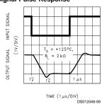
Non-Inverting Large Signal Pulse Response
