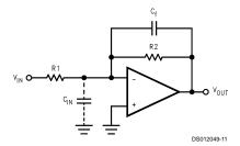
FIGURE 4. Cancelling the Effect of Input Capacitance
