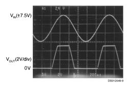
FIGURE 2. A ±7.5V Input Signal Greatly Exceeds the 5V Supply in Figure 3 Causing No Phase Inversion Due to R<sub>1</sub>
