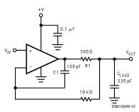
FIGURE 5. LMC6492/4 Noninverting Amplifier, Compensated to Handle Capacitive Loads
