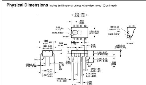
8-Lead (0.300" Wide) Molded Dual-In-Line Package Order Number LMC6492AEN or LMC6492BEN NS Package Number N08A
