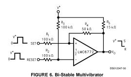
A bi-stable multivibrator has two stable states. The reference voltage is set up by the voltage divider of R<sub>2</sub> and R<sub>3</sub>. A pulse applied to the SET terminal will switch the output of the comparator high. The resistor divider of R<sub>1</sub>, R<sub>4</sub>, and R<sub>5</sub> now clamps the non-inverting input to a voltage greater than the reference voltage. A pulse applied to RESET will now toggle the output low.
