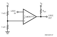
FIGURE 4. Universal Logic Level Shifter
