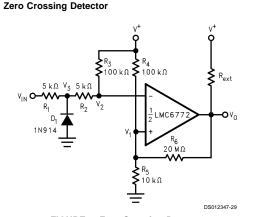
FIGURE 7. Zero Crossing Detector
