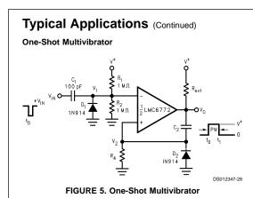
A monostable multivibrator has one stable state in which it can remain indefinitely. It can be triggered externally to another quasi-stable state. A monostable multivibrator can thus be used to generate a pulse of desired width.
