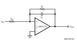
FIGURE 3. Canceling the Effect of Input Capacitance
