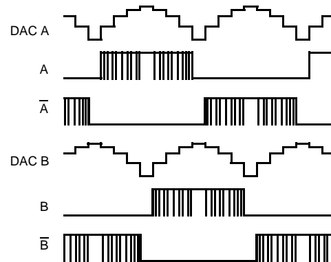
Figure 11: Stepper Motor Waveform - LM9833 Signals
