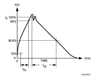
FIGURE 2. HBM Waveform
