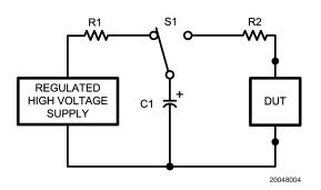
FIGURE 1. HBM ESD Test Model
