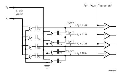
FIGURE 5. The Capacitive Voltage Divider
