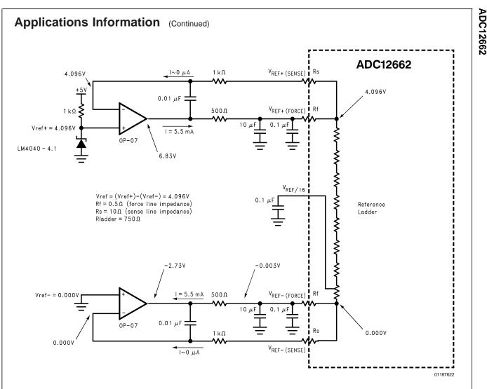
FIGURE 10. Reference Ladder Force and Sense Inputs
