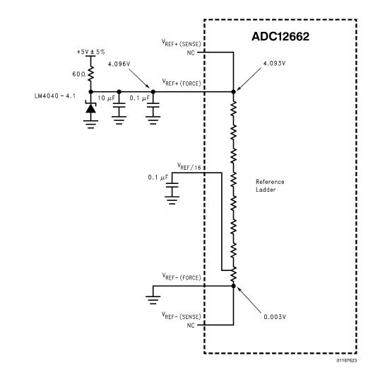
FIGURE 11. Using the V<sub>REF</sub> Force Pins Only
