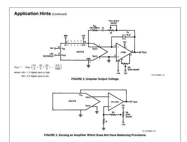
The selected amplifier should have as low an input bias current as possible since input bias current contributes to the current flowing through the feedback resistor. BI-FETTM op amps such as the LF356 or LF351 or bipolar op amps with super  $\beta$  input transistors like the LM11 or LM308A produce negligible errors.
