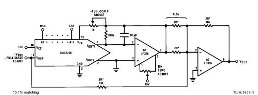
FIGURE 7. Obtaining a Bipolar Output from a Fixed Reference
