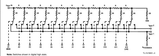
FIGURE 1. The R-2R Current Switching Ladder Network
