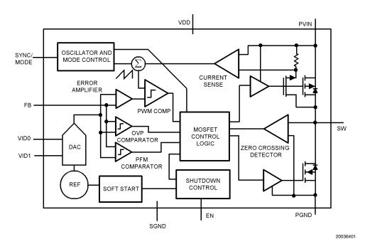
FIGURE 2. Simplified Functional Diagram
