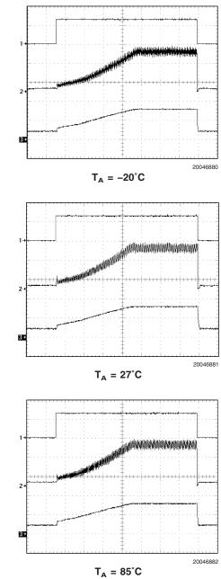
When programming the softstart time externally, simply use the equation given in the *Soft-Start Capacitor* section above. This equation uses the typical room temperature value of the soft start current,  $11\mu$ A, to set the soft start time.
