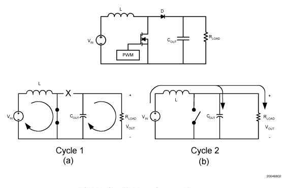
FIGURE 1. Simplified Boost Converter Diagram (a) First Cycle of Operation (b) Second Cycle Of Operation
