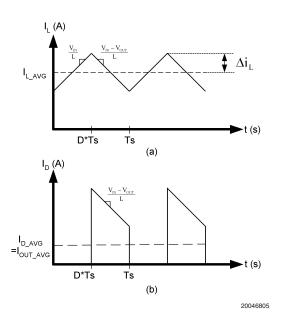
FIGURE 2. (a) Inductor current. (b) Diode current.
