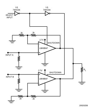
FIGURE 5. 2:1 MUX Operating off a 2.7V Single Supply
