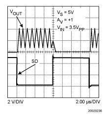
FIGURE 4. Output Held Low by Active Pull-Down Circuit
