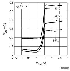
$V_{OS}$ vs.  $V_{CM}$  (A Typical Unit)
