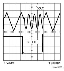
FIGURE 6. 2:1 MUX Output
