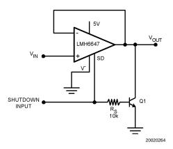
FIGURE 3. Active Pull-Down Schematic
