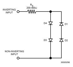
FIGURE 2. LMH6647 Equivalent Input in Shutdown Mode
