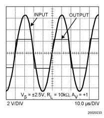
FIGURE 1. Input/Output Shown with Exceeded Input CMVR
