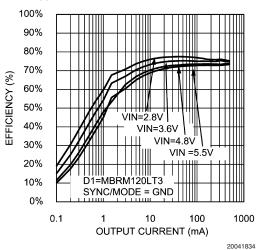
Efficiency vs Output Current (V<sub>OUT</sub> = 1.3V, PWM Mode, With Diode)
