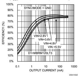
Efficiency vs Output Current (V<sub>OUT</sub> = 1.05V, PFM Mode, With Diode)
