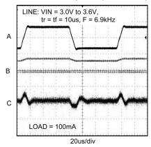
A: SUPPLY VOLTAGE, 500mV/div, AC COUPLED
