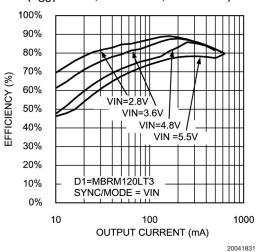
Efficiency vs Output Current (V<sub>OUT</sub> = 1.05V, PWM Mode, With Diode)
