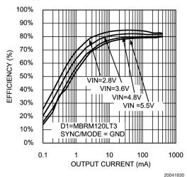
Efficiency vs Output Current (V<sub>OUT</sub> = 1.3V, PFM Mode, With Diode)
