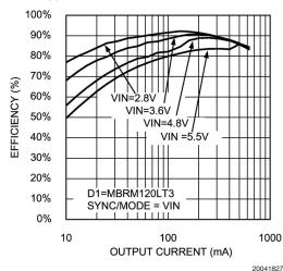
Efficiency vs Output Current (V<sub>OUT</sub> = 1.5V, PWM Mode, With Diode)
