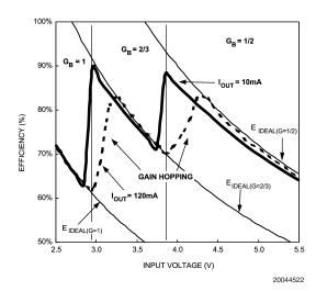
FIGURE 1. Efficiency of LM2798-1.8 with 10mA and 120mA output currents. Base-gain ( $G_B$ ) regions are separated and labeled. Ideal efficiency curves of charge pumps with G =1/2, 2/3, and 1 are included, and are labelled:
