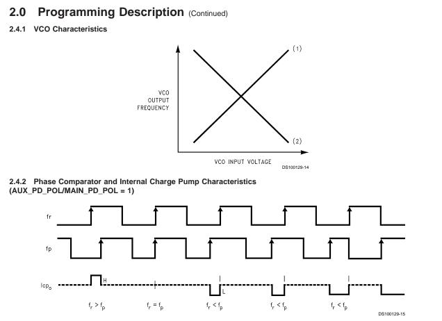
Note 15: fr is phase detector input from reference counter. fp is phase detector input from programmable N counter. Phase difference detection range:  $-2\pi$  to  $+2p\pi$ .
