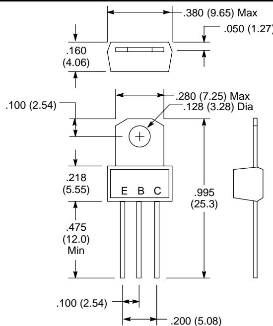
Collector Connected to Tab
