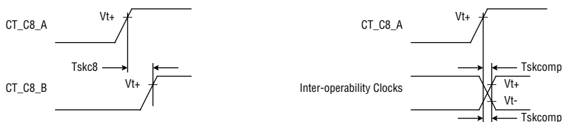
Figure 15. Clock Skew Requirements
