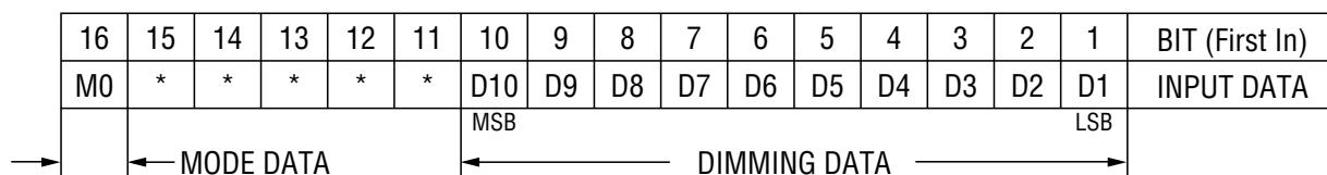
**[Input Configuration]****● Dimming data**
