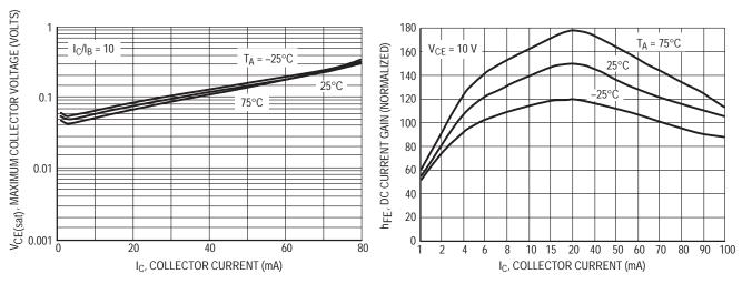
Figure 18. V<sub>CE(sat)</sub> versus I<sub>C</sub>
