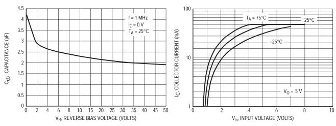
Figure 20. Output Capacitance
