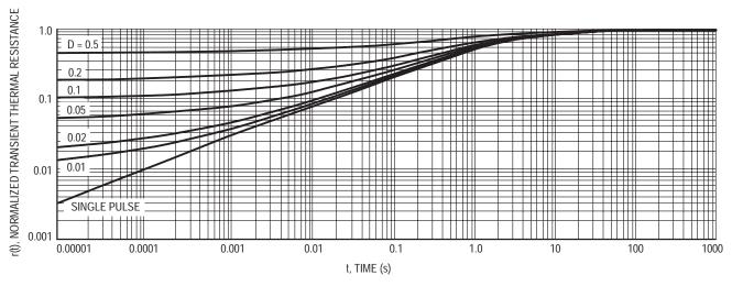
Figure 2. Normalized Thermal Response
