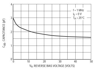
Figure 5. Output Capacitance
