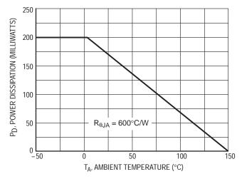
Figure 1. Derating Curve
