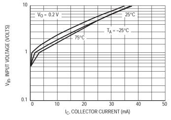
Figure 22. Input Voltage versus Output Current
