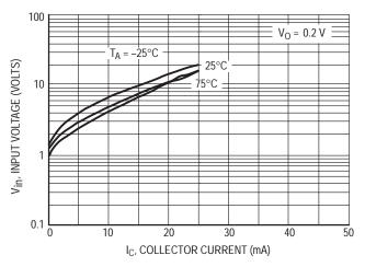
Figure 17. Input Voltage versus Output Current
