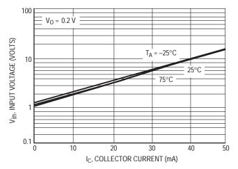
Figure 7. Input Voltage versus Output Current
