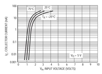
Figure 6. Output Current versus Input Voltage
