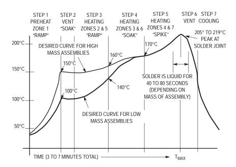
Figure 24. Typical Solder Heating Profile
