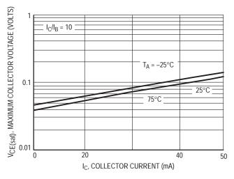
Figure 3. V<sub>CE(sat)</sub> versus I<sub>C</sub>
