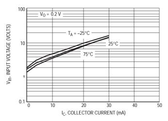
Figure 12. Input Voltage versus Output Current
