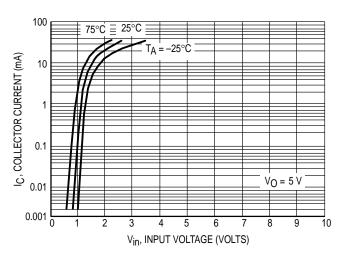
Figure 10. Output Current versus Input Voltage
