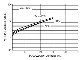
Figure 11. Input Voltage versus Output Current
