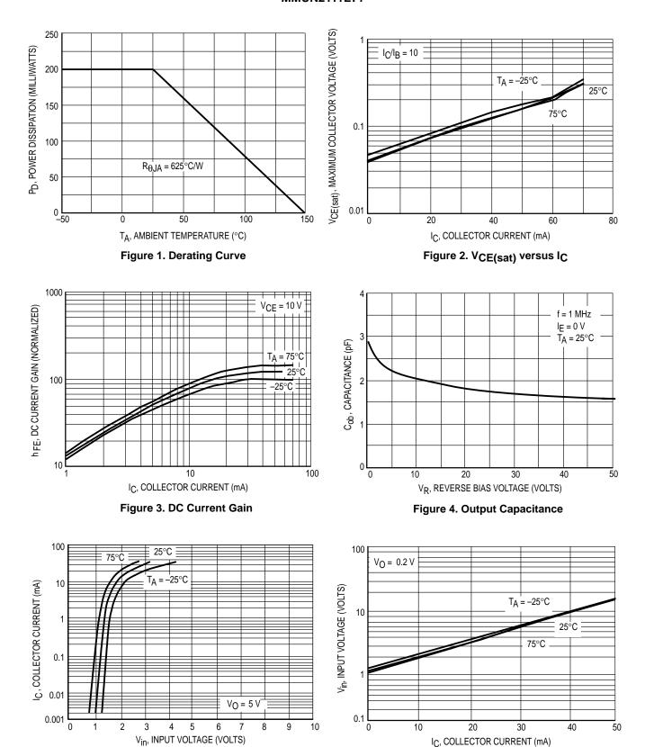
Figure 6. Input Voltage versus Output Current
