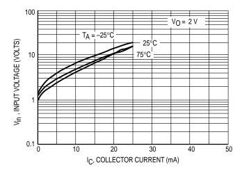
Figure 16. Input Voltage versus Output Current
