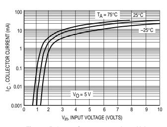
Figure 15. Output Current versus Input Voltage
