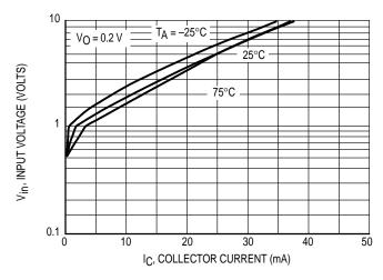
Figure 21. Input Voltage versus Output Current
