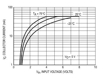
Figure 20. Output Current versus Input Voltage
