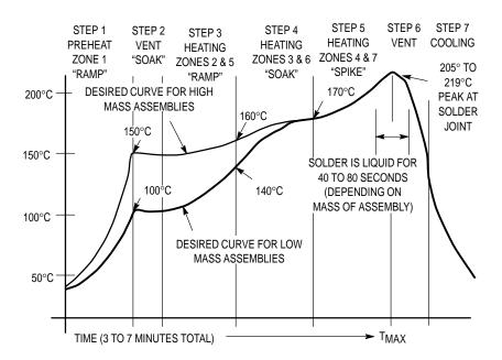
Figure 23. Typical Solder Heating Profile
