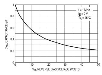
Figure 14. Output Capacitance
