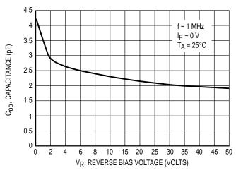
Figure 19. Output Capacitance
