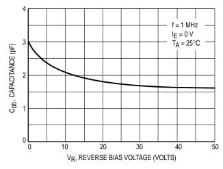
Figure 9. Output Capacitance
