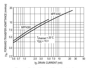
Figure 6. Typical Forward Transfer Admittance
