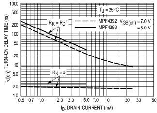
Figure 1. Turn-On Delay Time
