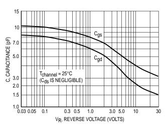
Figure 7. Typical Capacitance
