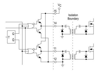
Figure 32. Bipolar Transistor Drive
