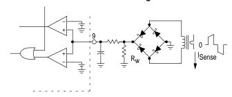
The addition of an RC filter will eliminate instability caused by the leading edge spike on the current waveform. This sense signal can also be used at the ramp input pin for current mode control. For ramp compensation it is necessary to know the gain of the current feedback loop. The gain can be calculated by:
