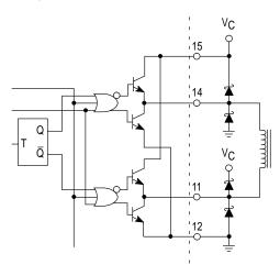
The totem pole output can easily drive pulse transformers. A Schottky diode is recommended when driving inductive loads at high frequencies. The diode can reduce the driver's power dissipation due to excessive ringing, by preventing the output pin from being driven below ground.
