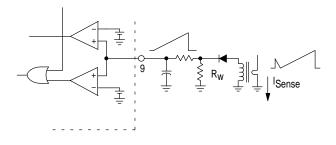
Figure 27. Primary or Secondary Side Current Sensing
