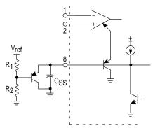
In voltage mode operation, the maximum duty cycle can be clamped. By the addition of a PNP transistor to buffer the clamp voltage, the Soft–Start current is not affected by  $R_1$ .
