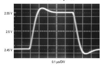
Figure 6. Error Amp Large Signal **Transient Response**
