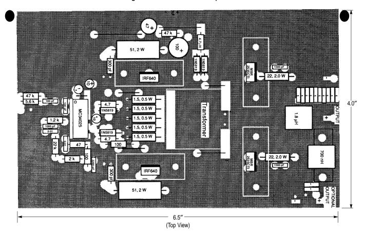
Figure 38. PC Board Without Components
