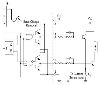
The totem pole output can furnish negative base current for enhanced transistor turn-off, with the addition of the capacitor in series with the base.
