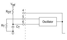
Additional dead time can be added by the addition of a dead time resistor from  $V_{ref}$  to  $C_T$ . See text on oscillator section for more information.
