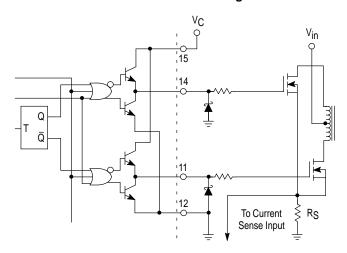
A series gate resistor may be needed to damp high frequency parasitic oscillation caused by a MOSFET's input capacitance and any series wiring inductance in the gate–source circuit. The series resistor will also decrease the MOSFET's switching speed. A Schottky diode can reduce the driver's power dissipation due to excessive ringing, by preventing the output pin from being driven below ground. The Schottky diode also prevents substrate injection when the output pin is driven below ground.
