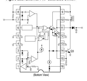
Figure 24. Voltage–Inverting Converter
