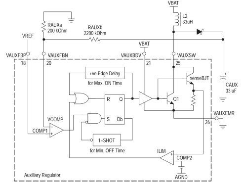
Figure 21. Simplified Block Diagram of Auxiliary Regulator
