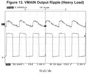
1: VMAIN = 3.3 V (50 mV/div, AC COUPLED) 2: Voltage at VMAINSW (1 V/div)
