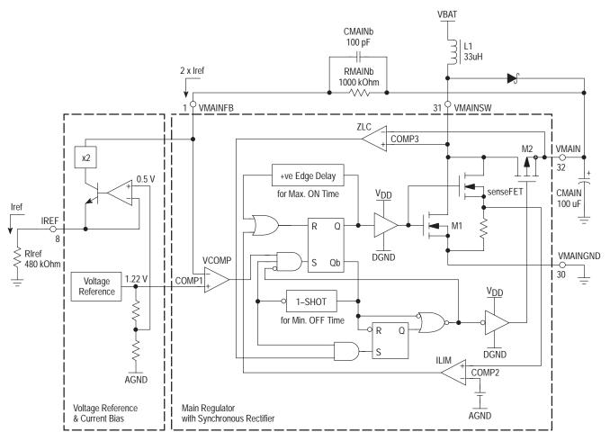
Figure 18. Simplified Block Diagram of Main Regulator
