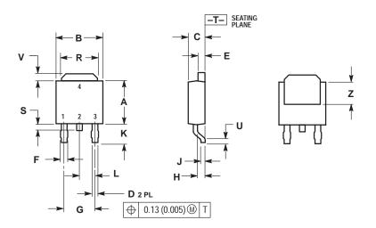
NOTES: 1. DIMENSIONING AND TOLERANCING PER ANSI Y14.5M, 1982. 2. CONTROLLING DIMENSION: INCH.
