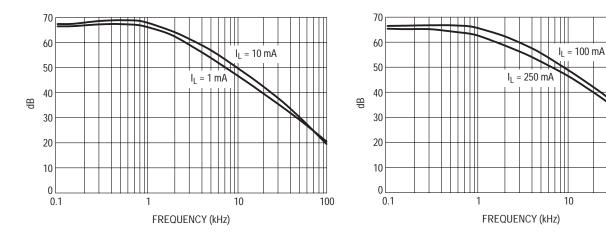
Figure 13. Ripple Rejection
