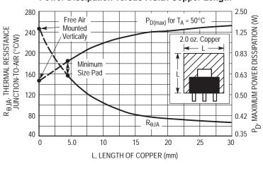
Figure 16. SOT–223 Thermal Resistance and Maximum Power Dissipation versus P.C.B. Copper Length
