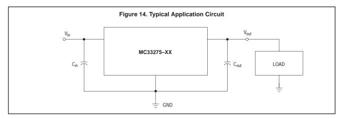
The MC33275 regulators are designed with internal current limiting and thermal shutdown making them user-friendly. Figure 14 is a typical application circuit. The output capability of the regulator is in excess of 300 mA, with a typical dropout voltage of less than 260 mV. Internal protective features include current and thermal limiting.
