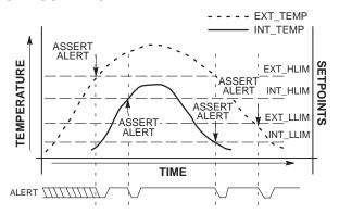
Note: This diagram implies that the appropriate setpoint is moved, temporarily, after each ALERT event to suppress re–assertion of ALERT immediately after the ARA/de–assertion.
