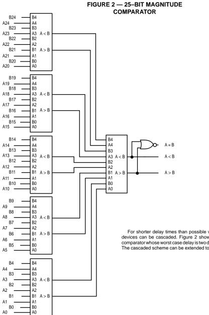
For shorter delay times than possible with serial expansion, devices can be cascaded. Figure 2 shows a 25-bit cascaded comparator whose worst case delay is two data-to-output delays. The cascaded scheme can be extended to longer word lengths.
