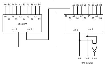
For longer word lengths, the MC10H166 can be serially expanded or cascaded. Figure 1 shows two devices in a serial expansion for a 9–bit word length. The A > B and A < B outputs are fed to the A0 and B0 inputs respectively of the next device. The connection for an A = B output is also shown. The worst case delay time of serial expansion is equal to the number of comparators times the data-to-output delay.
