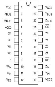
Pin assignment is for Dual–in–Line Package. For PLCC pin assignment, see the Pin Conversion Tables on page 6–11 of the Motorola MECL Data Book (DL122/D).
