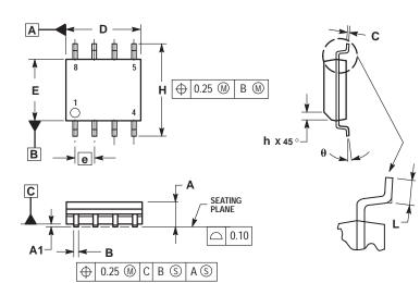
NOTES: 1. DIMENSIONING AND TOLERANCING PER ASME Y14.5M, 1994. 2. DIMENSIONS ARE IN MILLIMETER. 3. DIMENSION D AND E DO NOT INCLUDE MOLD PROTRUSION. 4. MAXIMUM MOLD PROTRUSION 0.15 PER SIDE. 5. DIMENSION B DOES NOT INCLUDE DAMBAR PROTRUSION. ALLOWABLE DAMBAR PROTRUSION SHALL BE 0.127 TOTAL IN EXCESS OF THE B DIMENSION AT MAXIMUM MATERIAL CONDITION.
