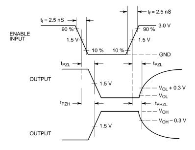
Figure 5. Enable/Disable Delays
