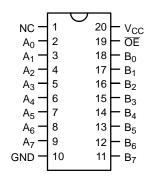
Figure 1. 20-Lead Pinout
