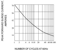
Fig. 3-FORWARD CURRENT DERATING CURVE
