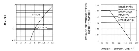
Fig. 2-FORWARD CHARACTERISTICS
