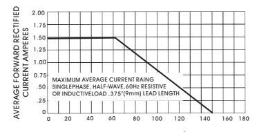
AMBIENT TEMPERATURE, °C Fig. 3-FORWARD DERATING CURVE
