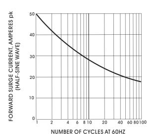
Fig. 2-MAXIMUM OVERLOAD SURGE-CURRENT
