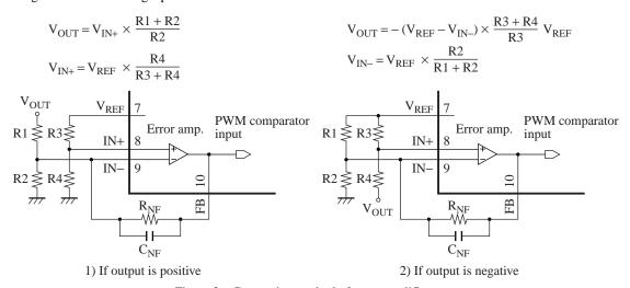
Figure 3. Connection method of error amplifier
