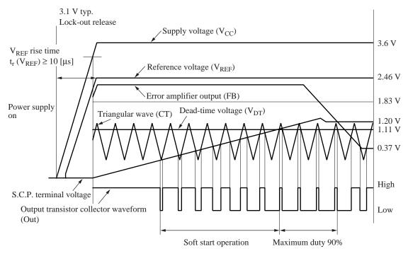
Figure 1. PWM comparator operation waveform
