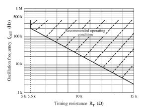
Figure 5. Timing resistance recommended condition
