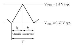
Figure 4. Triangular wave oscillation waveform
