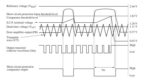
Figure 2. Short-circuit protection operation waveform
