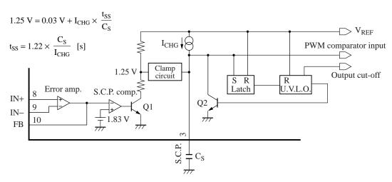
Figure 6. Short-circuit protection circuit
