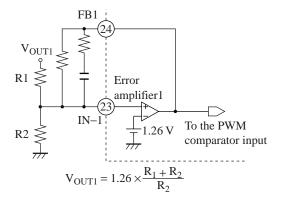
Figure 2. Connection method of error amplifier 1 (Step-up output)
