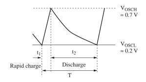
Figure 1. Triangular oscillator waveform
