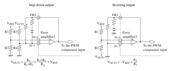
Figure 4. Connection method of error amplifier 3
