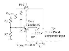
Figure 3. Connection method of error amplifier 2 (Step-up output)
