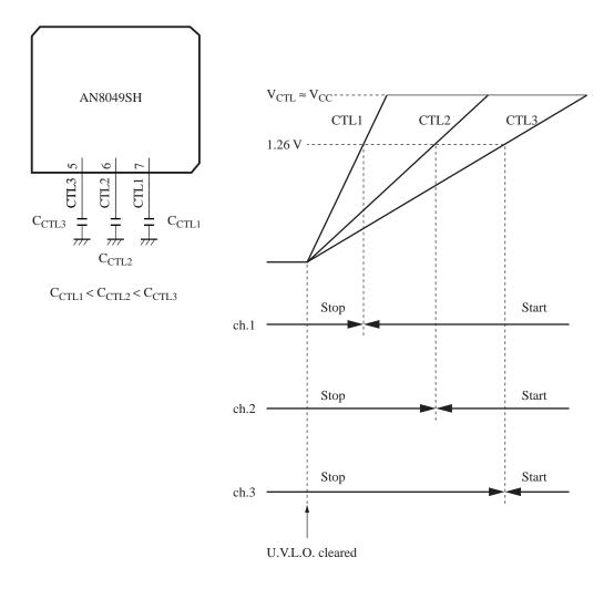
Figure 8. Sequential operation using external capacitors
