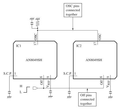
Figure 7. Synchronous parallel operation
