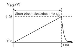
Figure 5. S.C.P. pin charging waveform
