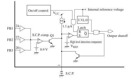
Figure 6. Short-circuit protection circuit
