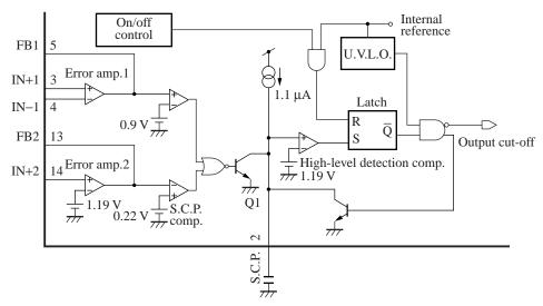
Figure 6. Short-circuit protection circuit
