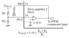
Figure 3. Connection method of error amplifier 2 block (step-up output)
