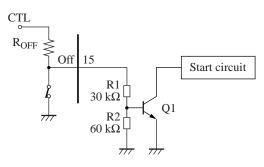
Figure 9. Off terminal peripheral circuit
