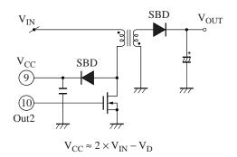
Figure 2. Gate drive voltage increasing method
