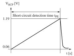
Figure 5. S.C.P. terminal charging waveform
