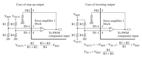
Figure 2. Connection method of error amplifier 1 block
