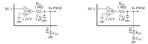
Figure 11. Error amplifier equivalent circuit
