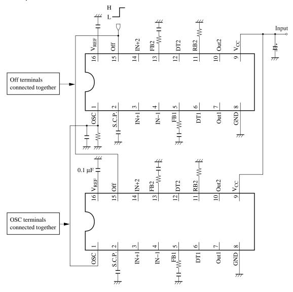
Figure 7. Slave operation circuit example
