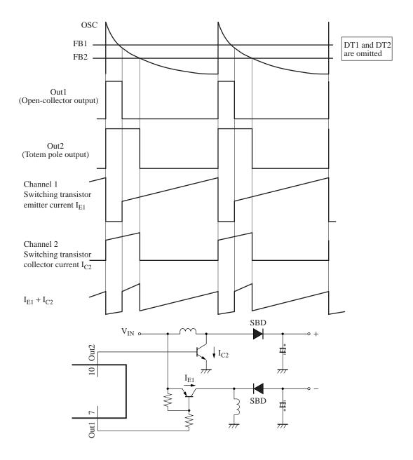
Figure 4. PWM logic explanation chart
