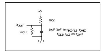
Figure 1. Output Load
