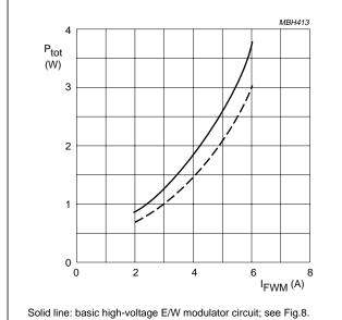
Dotted line: basic conventional horizontal deflection circuit; see Fig.9. Curves include power dissipation due to switching losses.
