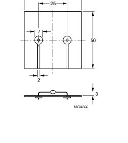
Fig.19 Device mounted on a printed-circuit board.
