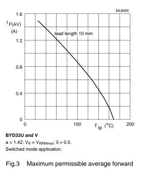
current as a function of tie-point temperature (including losses due to reverse leakage).
