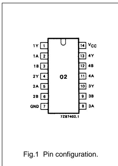
Fig.1 Pin configuration.
