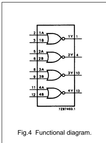
Fig.4 Functional diagram.
