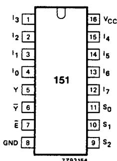
Fig.1 Pin configuration.
