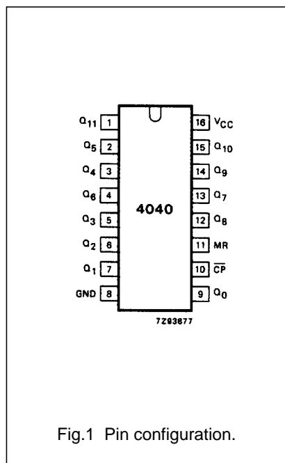
Fig.1 Pin configuration.
