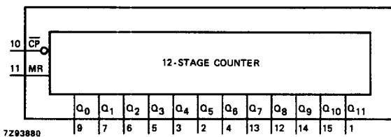
Fig.4 Functional diagram.
