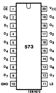
Fig.1 Pin configuration.
