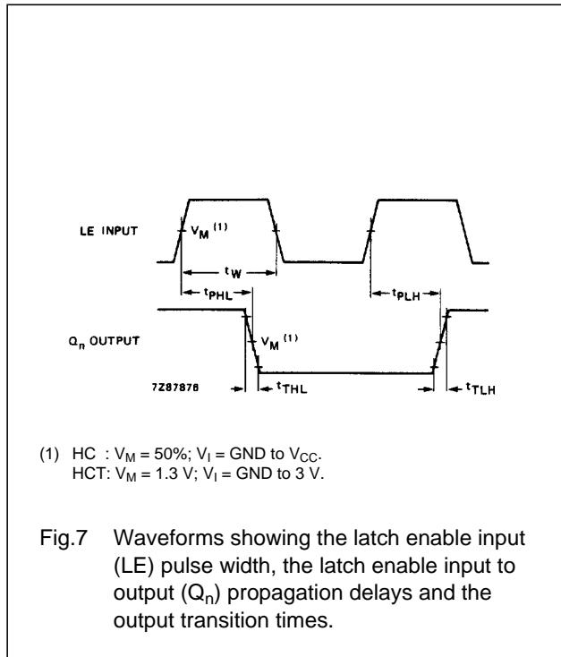
Fig.7 Waveforms showing the latch enable input (LE) pulse width, the latch enable input to output ( $Q_n$ ) propagation delays and the output transition times.
