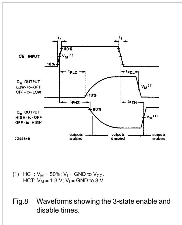
Fig.8 Waveforms showing the 3-state enable and disable times.
