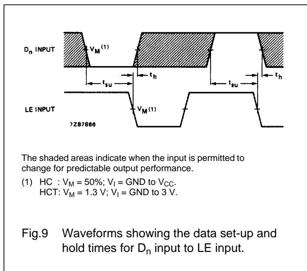
Fig.9 Waveforms showing the data set-up and hold times for  $D_n$  input to LE input.
