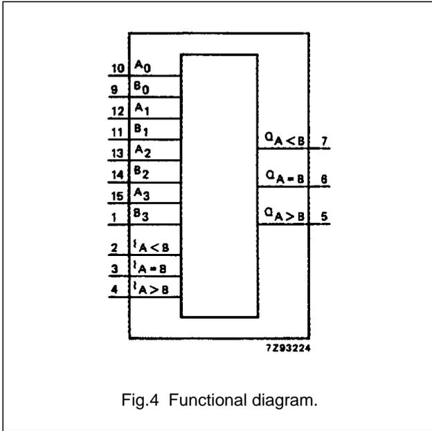
Fig.4 Functional diagram.
