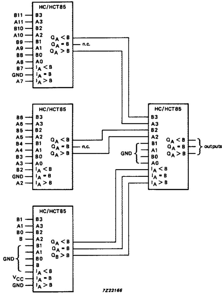
Fig.8 Parallel cascading; comparing 12-bit words.
