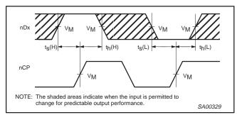
Waveform 2. Data Setup and Hold Times
