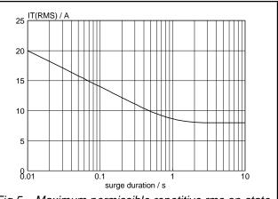
Fig.5. Maximum permissible repetitive rms on-state current  $I_{T(RMS)}$ , versus surge duration, for sinusoidal currents, f = 50 Hz;  $T_{mb} \le 102^{\circ}C$ .
