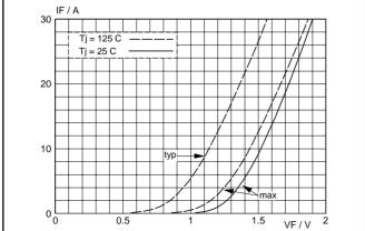
Fig.5. BY329-1500 Typical and maximum forward characteristic  $I_F = f(V_F)$ ; parameter  $T_j$
