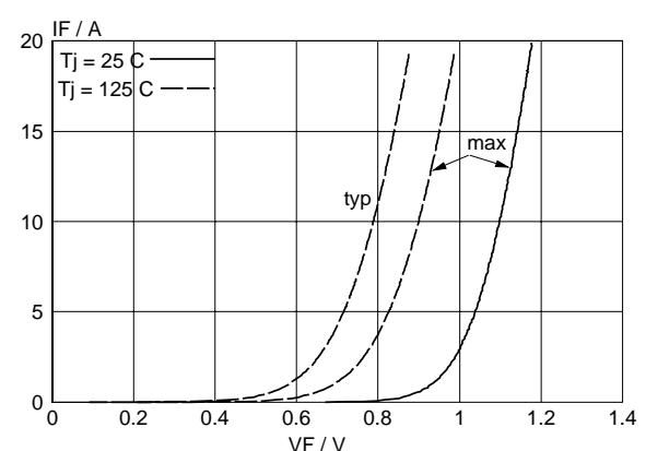
Fig.4. Typical and maximum forward characteristic
