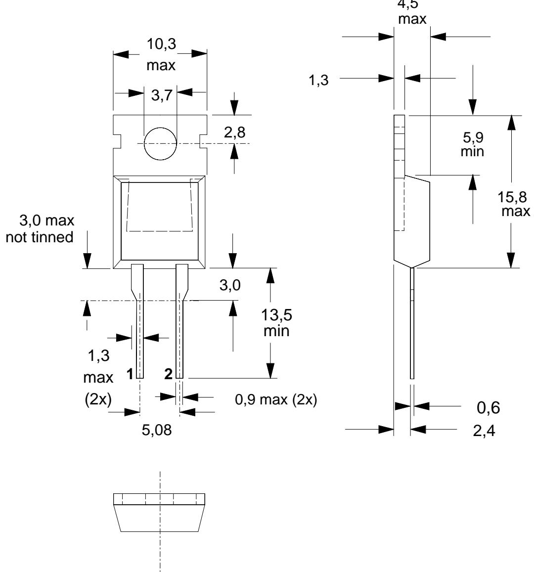
Fig.7. SOD59 (TO220AC). pin 1 connected to mounting base.
