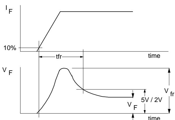
Fig.1. Definition of  $V_{fr}$  and  $t_{fr}$
