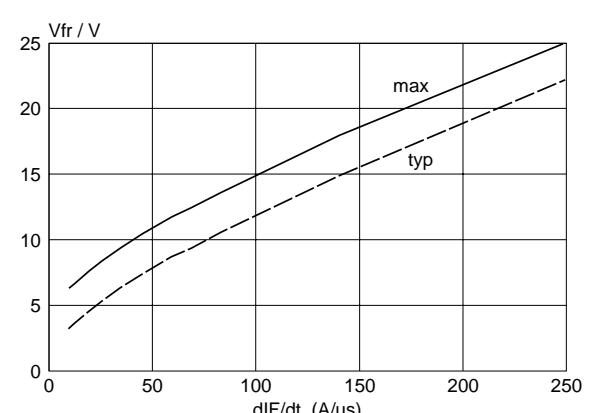
Fig.5. Typical and maximum  $V_{fr} = f(dI_F/dt)$ ;  $I_F = 10 \text{ A}$ ;  $T_j = 25^\circ\text{C}$
