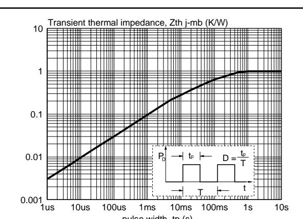
Fig.6. Transient thermal impedance  $Z_{th} = f(t_p)$
