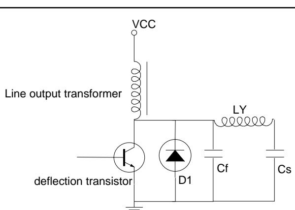
Fig.3. Basic horizontal deflection circuit.
