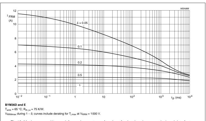
Fig.12 Maximum repetitive peak forward current as a function of pulse time (square pulse) and duty factor.
