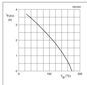
$a = 1.42; \ V_R = V_{RRMmax}; \ \delta = 0.5.$  Switched mode application.
