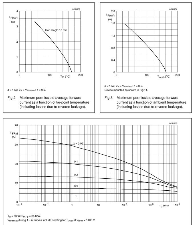
Fig.4 Maximum repetitive peak forward current as a function of pulse time (square pulse) and duty factor.
